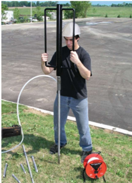
Figure 15 and 16) left: drive-point piezometer components and set-up, right: drive-hammer operation
