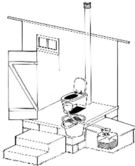
Figure 2.7 – Small-scale urine-diverting collection system
