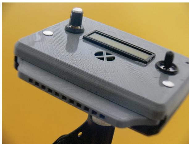
Fig. 3.22 – A current version of the XHarp , a device presented in Read and Hebert (2013). Photo courtesy of Wayne Read.
