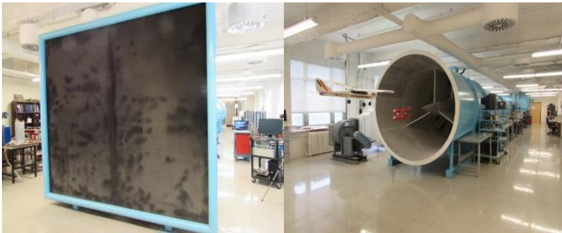
Figure 14 top) Schematic diagram of wind tunnel bottom left) Inlet of the wind tunnel, and bottom right) acoustic silencer of the wind tunnel
