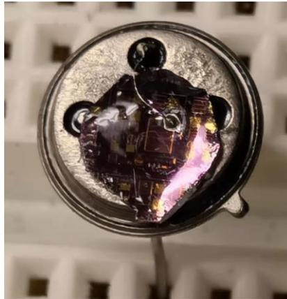
Figure 22: Image of encapsulated AlGaN nanowire DUV LED die.
