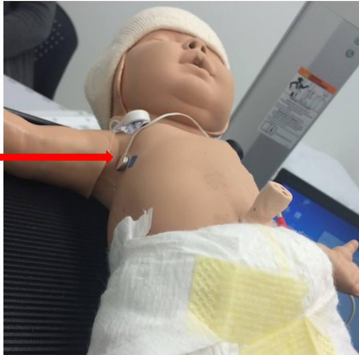
Figure 4.5. Setup showing placement of the temperature probe under the axilla of the patient. Temperature probe should be secured using a sticker with the white plastic side of the probe in good physical contact with the skin during recordings.
