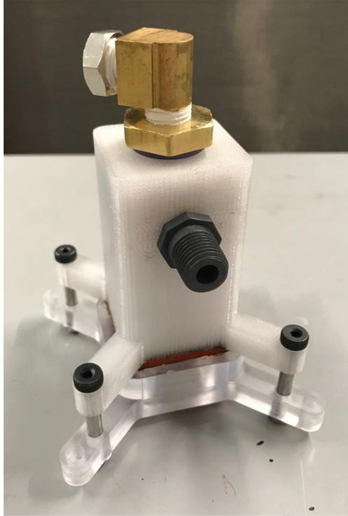
Figure 3-9: Spray chamber assembled - top isometric view.
