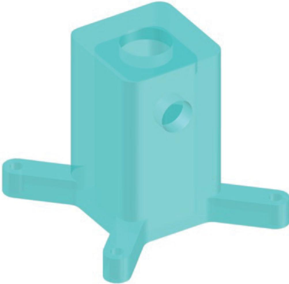
Figure 3–8: Spray chamber lid - CAD - top isometric view.
