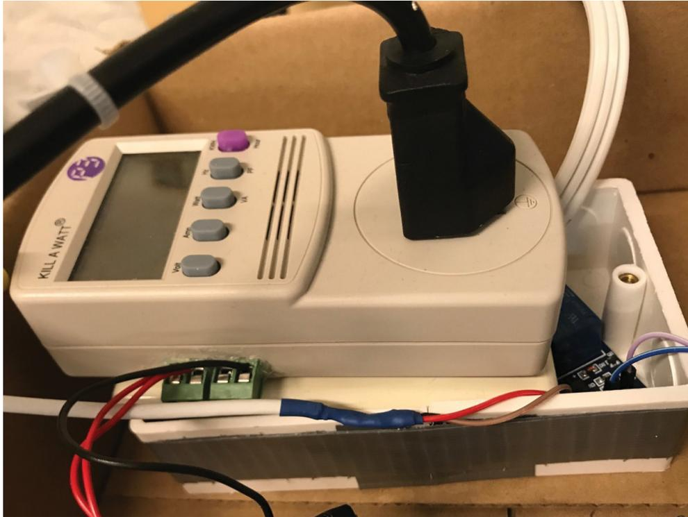
Figure 2-6: Modified Kill A Watt Electricity Usage Monitor attached to custom breaker outlet.
