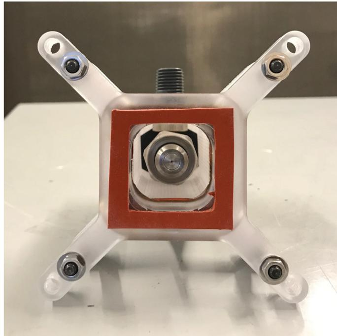
Figure 3-10: Spray chamber assembled - bottom view.
