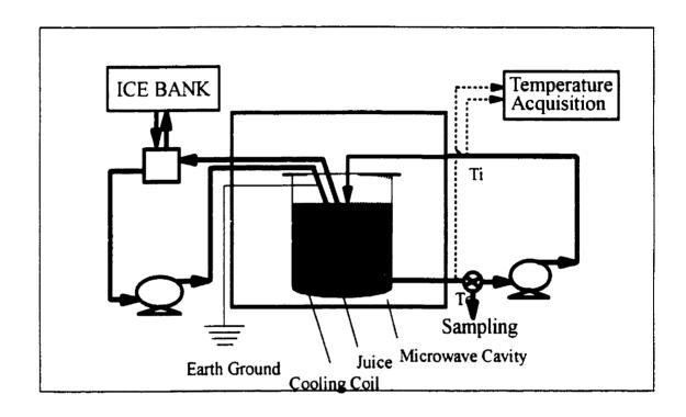
Figure 7.2 A schematic diagram of batch-mode microwave heating for evaluation of non-thermal effects at low temperatures.
