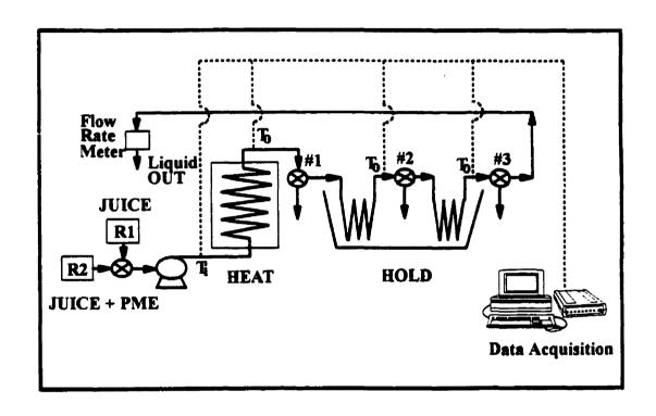
Figure 4.1 A schematic diagram of continuous-flow microwave heating and isothermal holding system set-up.
