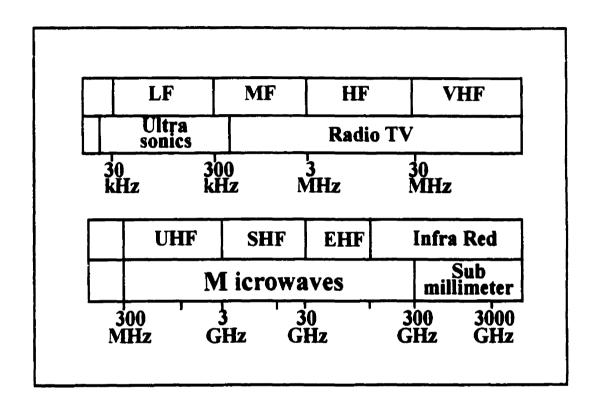
Figure 2.1 Electromagnetic spectrum (Source: Decareau and Peterson, 1986).
