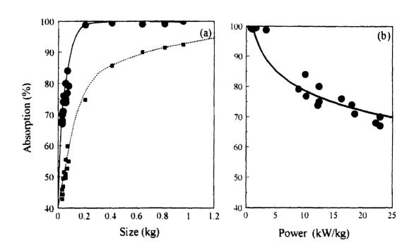
Figure 7.15 Percentage of microwave energy absorption as a function of (a) size at 700 W microwave power and (b) power for unit mass (kW/kg).
