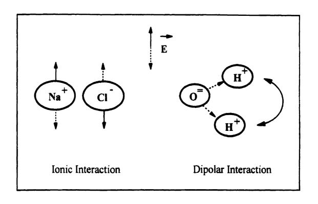
Figure 2.2 Microwave heating mechanisms (Source: Buffler, 1993).
