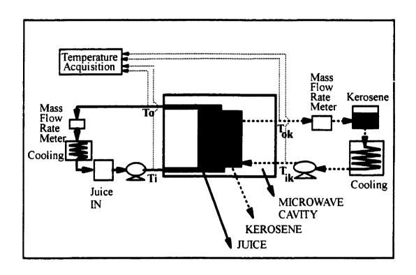
Figure 7.1 A schematic diagram of continuous-flow microwave heating system for evaluation of non-thermal effects at low temperatures.
