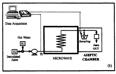
Figure 5.1 Schematic diagrams of continuous-flow microwave heating systems (a) enzyme inactivation in orange juice and (b) microbial destruction in apple juice.
