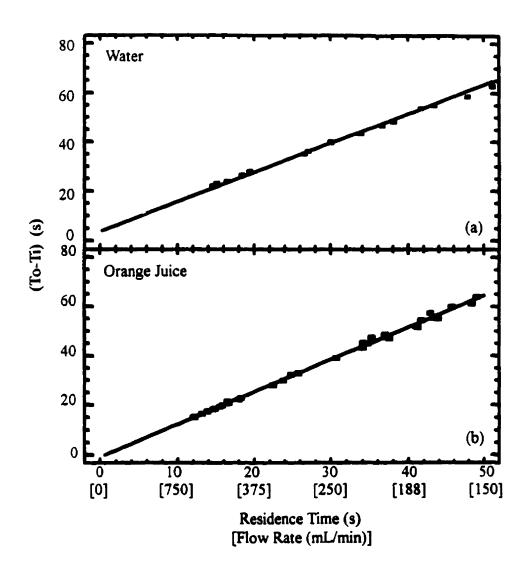
Figure 4.3 Temperature rise for (a) water and (b) orange juice as a function of residence time [flow rate] (125 mL heating volume).
