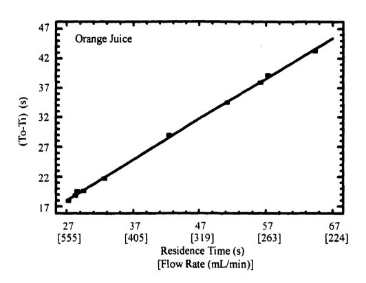
Figure 4.4 Temperature rise for orange juice as a function of residence time [flow rate] (250 mL heating volume).
