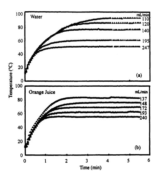
Figure 4.2 Microwave heating curves for (a) water and (b) orange juice as a function of flow rate.
