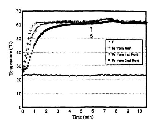
Figure 4.5 Temperature of orange juice during continuous-flow microwave heating and isothermal holding at 251 mL/min (125 mL heating volume).
