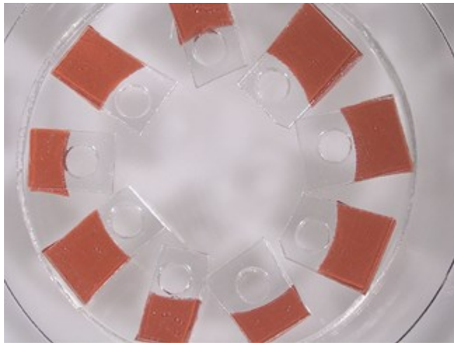
Fig. 2.7. Multiple mounting stages to image more than one embryo in the same experiment. The use of a larger glass microwell (35mm petri dishes) enables the imaging of multiple embryos during the same experiment. For this option to be effective, a microscope with a motorized stage is required.
