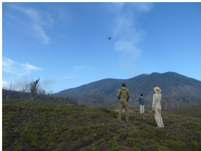
Figure 5: A drone equipped with compact gas instrumentation is flown toward the volcanic gas plume at Turrialba volcano in Costa Rica. Researchers are able to fly the drone from a safe distance while it measures key gases.
