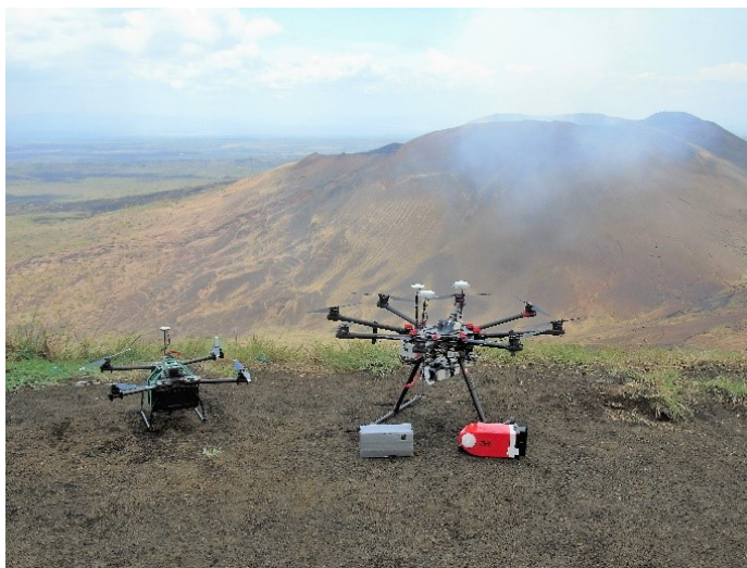
Figure 10: Masaya volcano, 6 May 2017. Left: A custom-built RAVEN (payload 1.3 kg) quadcopter with the denuder sampling unit mounted on board. Right: A DJI S1000 octocopter (payload 5.1 kg) with the DROAS unit in grey, and the MiniGAS unit in red, placed in front.
