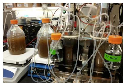
Figure 5 – Chemostat-based artificial GIT systems. (a) The SHIME system that is comprised of five vessels simulating the stomach, small intestine, and colon. Parameters such as anaerobiosis, mixing, pH control, and temperature are mimicked within each vessel, while the SHIME is able to support complex microbiota through culturing fecal matter. Adapted from Molly et al. [72]. (b) The TIM systems comprises of the TIM-1, which simulates the stomach and small intestine, and the TIM-2, which simulates the colon. Peristalsis motions can be mimicked, as well as absorption capacities similar to in vivo conditions through dialysis membranes modified in the vessels. Adapted from Verwei et al. and Minekus et al. [80, 81]. (c) The RoboGut system, which is composed of a single chemostat simulating the colon. Similar to the SHIME, the RoboGut can support complex microbiota through culturing fecal matter, while able to perform two experiments with the same sample simultaneously through multiplexing its chemostats (“twin-vessel”). Adapted from McDonald et al. [77].
