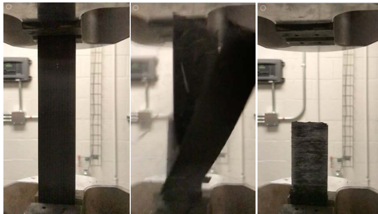
Figure 79 Tensile test failure in slow-motion
