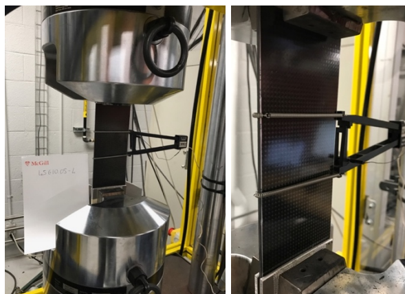
Figure 82 Extensometer used during tensile test
