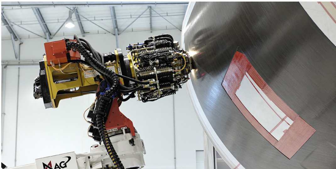
Figure 5 AFP machine laying down fibres on a mould at STELIA Aerospace 3
