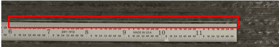
Figure 48 Half gap / half overlap unwanted defect
