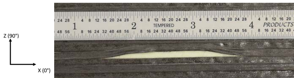
Figure 49 Defect manually created with Mylar sheet
