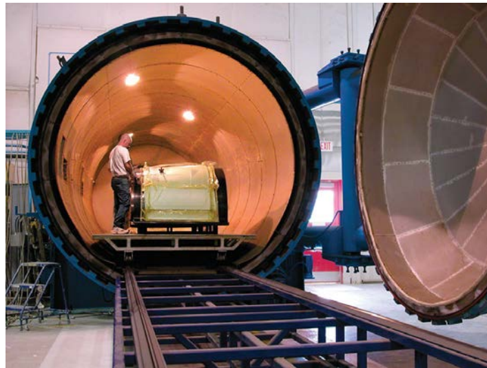
Figure 4 Autoclave of American Airlines' composite repair shop 2
