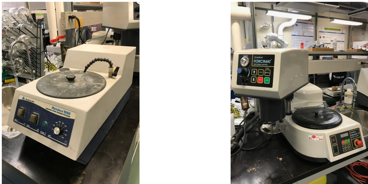
Figure 58 Manuel polisher 200-P grit on the left and automated polisher on the right
