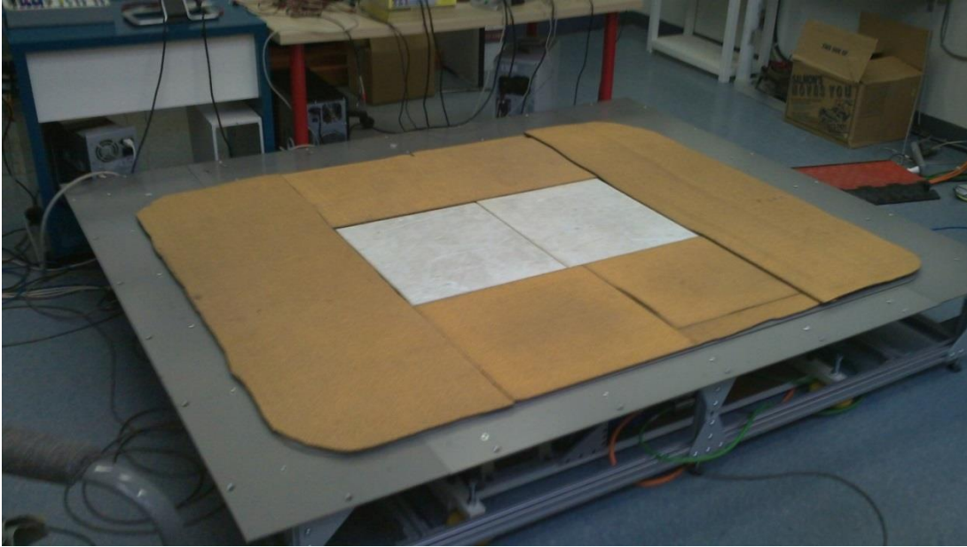
Figure 3: Perturbation platform with two embedded force plates (center). Each force plate has a polyethylene artificial ice surface adhered to the surface and is surrounded by protective rubber mats.
