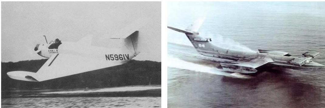
Figure 1–2: Early WIG crafts in the 1960s: Lippisch-type Collins X-112 of the US [2] (left), Ekranoplan-type KM of the USSR [3] (right).
