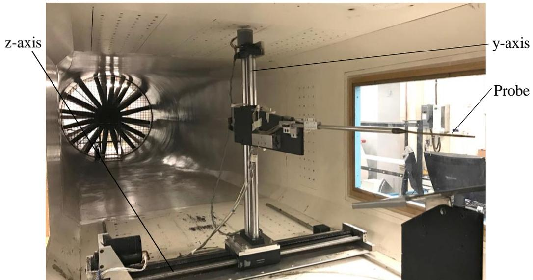
Figure 3-4: Seven-hole pressure probe and traverse mechanism. (a) schematic diagram of the probe [14]; (b) the traverse.
