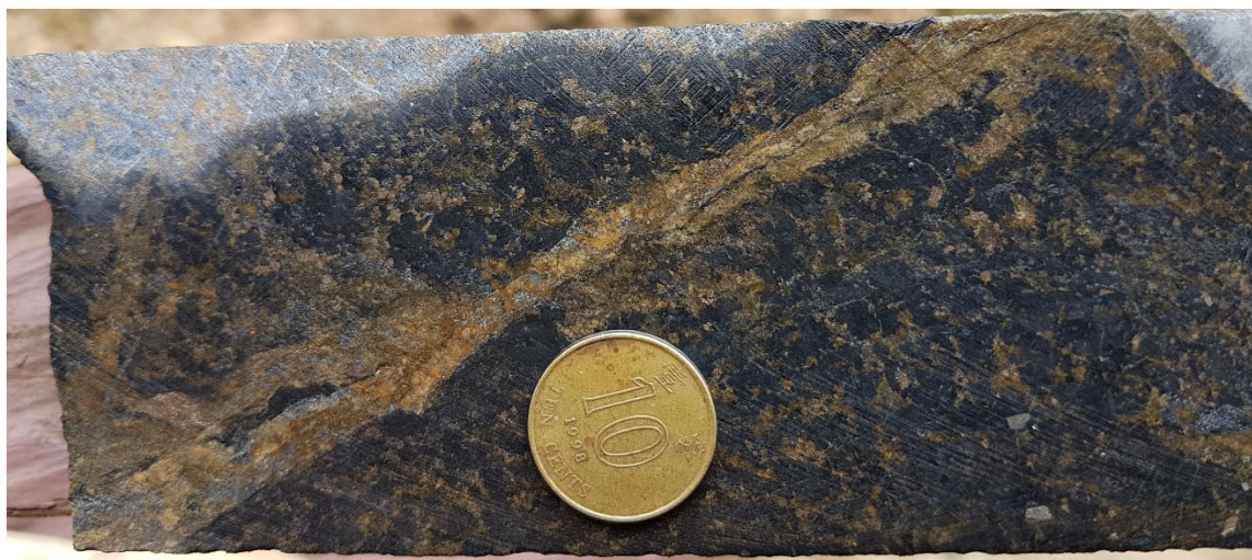
Figure 5: Disseminated and vein-hosted pyrrhotite and arsenopyrite in quartz diorite accompanied by pervasive ankeritic alteration in drill core from the Kibi-Gold Project.
