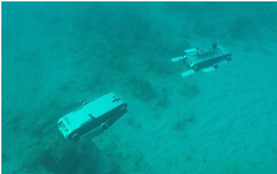
Figure 5–1: A convoy of two Aqua robots showcasing the typical view of a follower Aqua.
