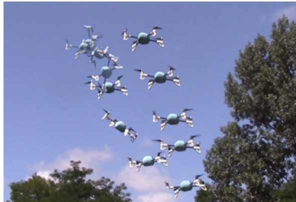
FIGURE 4.23: Quadrotor Rolling Flip Case 2 Image Sequence: The flip begins on the left side of the image, performs the flip quickly, loses altitude, and then returns to the start of the maneuver
