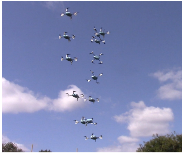
FIGURE 4.21: Quadrotor Rolling Flip Case 1 Image Sequence: The flip begins on the right side of the image, performs the flip while losing altitude, and then returns to the start of the maneuver
