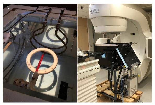
Figure 4.13: Experimental set-up for the adiabatic measurement. (A) The center of the probe (red) is placed at the center of a  $10 \times 10$  cm<sup>2</sup> jaw-defined field and at a depth of 10 cm in the water phantom. The adiabatic measurements were done with the phantom lid closed (lid shown in B hanging off the side of the phantom). (B) Overview of the temperature-controlled water phantom placed under the linear accelerator just before measurement.
