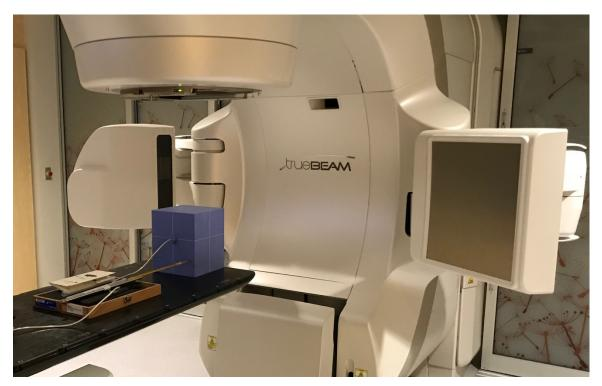
Figure 4.1: Photo of the setup for the first isothermal mode measurements performed on Nov 7th, 2018. The blue water equivalent phantom is placed at SSD 100 cm with its center aligned with the beam axis. The gantry is positioned at a 0° angle. In the center of the phantom, the detector is inserted in a dedicated sleeve to position the center of the core at a depth of 10 cm in phantom. A hole is drilled at the lower corner of the phantom to insert a thermometer.
