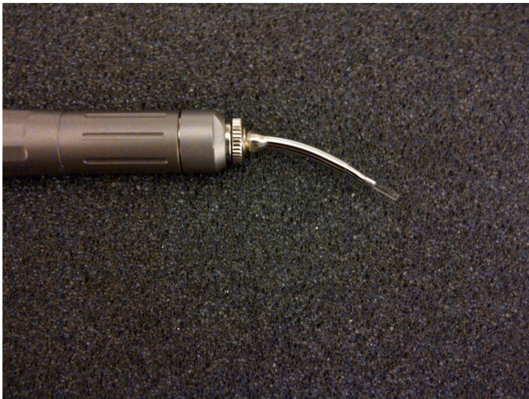
Figure 5-1: Glass fiber Er:YAG laser handpiece tip (800 \mu\text{m} ).
