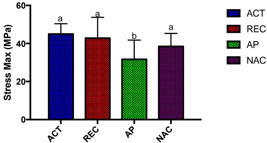
**FIGURE 29:** Strain Max of right femur determined by INSTRON in piglets with DSS induced colitis in the active phase (ACT) at day 10 and recovery phases (REC, AP, NAC) at day 15. Values are mean + SD, ACT n = 5 per group; REC, n = 5; AP, n = 6; NAC, n = 5. Means without a common superscript differ,  $p < 0.05$ .
