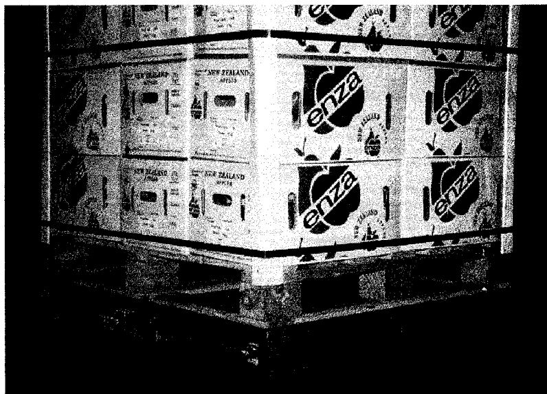
Figure 2.12: Produce loaded on a 4-way-double-deck-cube-beam pallet placed on top of a 4-way-double-deck-solid-beam pallet.
