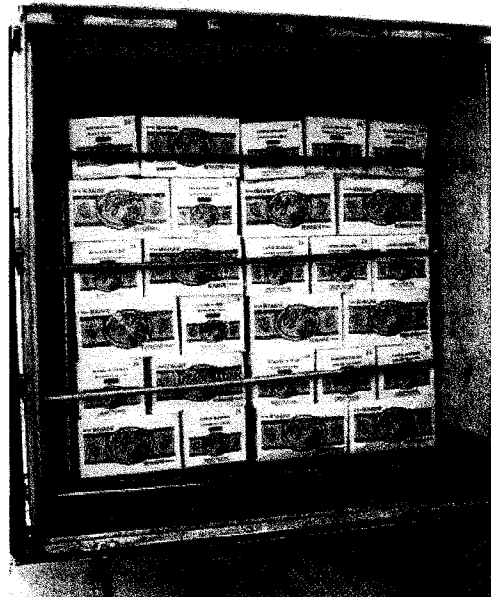
Figure 2.17: The use of lock bars to prevent produce from shifting backward.
