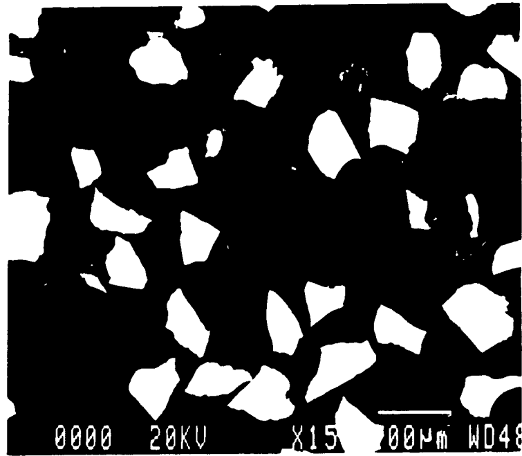
Figure 6.6 : SEM photograph of [75-106 \mu\text{m} grain/53-75 \mu\text{m} particle/doped Epofix] locked particles.
