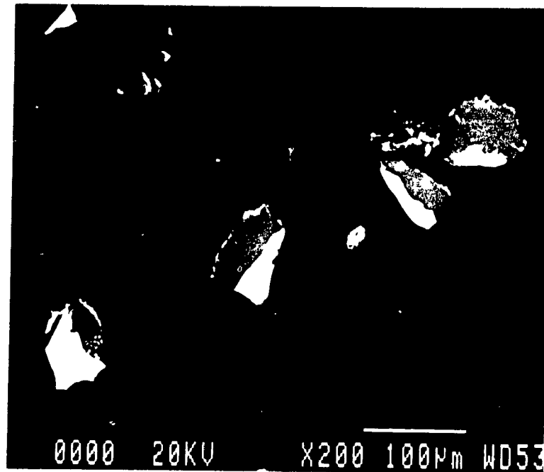
Figure 6.1 : SEM photograph of [600-850 \mu\text{m} grain/38-75 \mu\text{m} particle/doped Epofix] locked particles.
