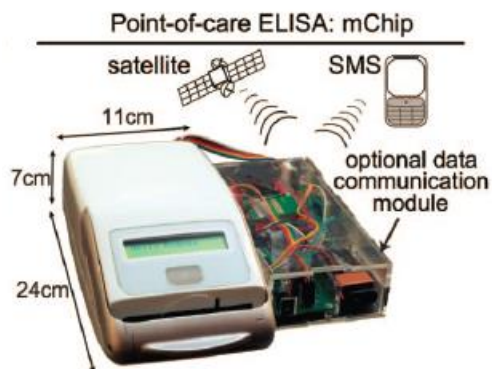
Figure 2.11: Overview of a microfluidic chip device with a wireless module for onsite ELISA
