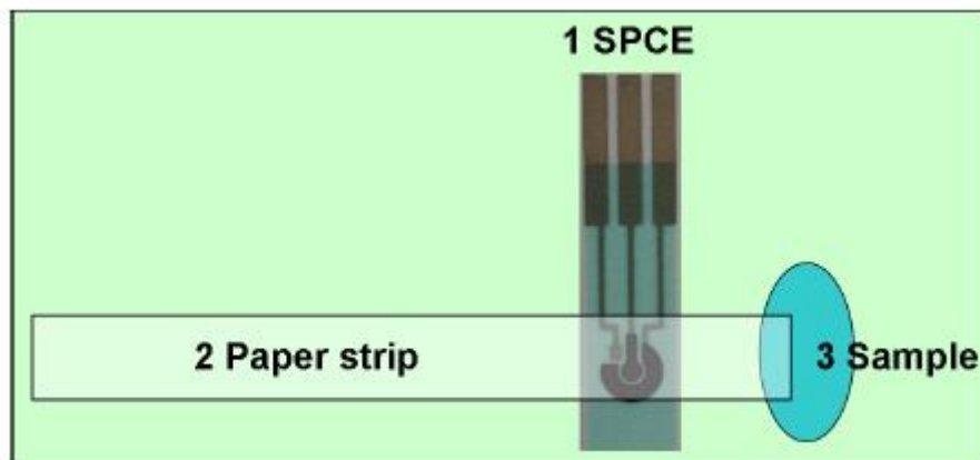
Figure 2.6: Schematic layout of a paper-based electrochemical sensing device. The sensor comprises (1) a screen-printed capillary electrode (SPCE), (2) a paper strip and (3) a sample cell.
