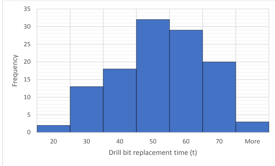
Figure 6-3: Histogram of the failure times of 123 rotary drill tri-cone rock roller bits
