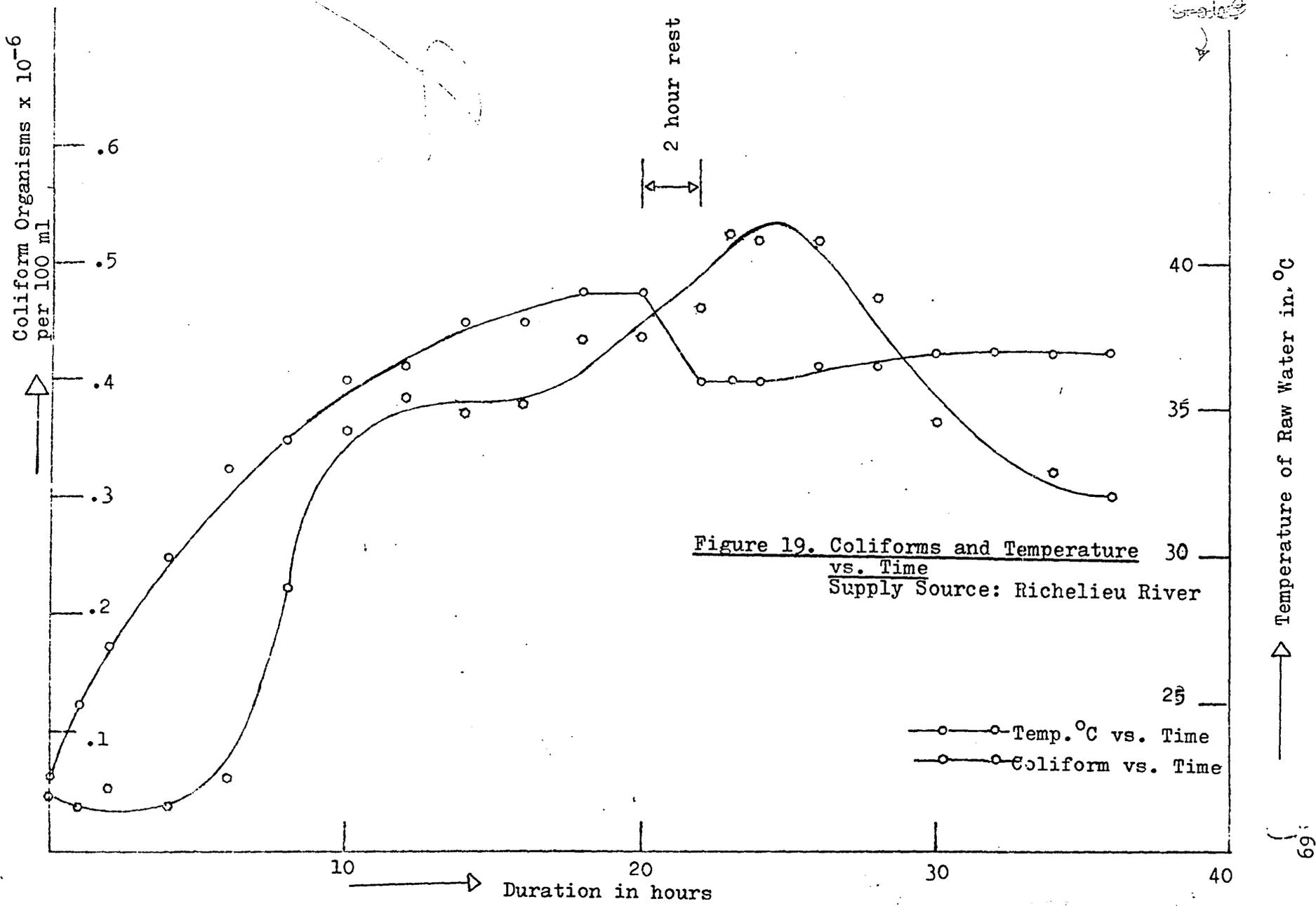
Figure 19. Coliforms and Temperature vs. Time
