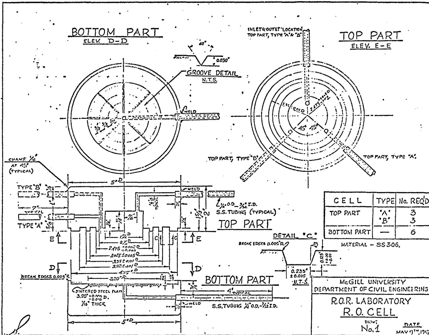
Figure 7. Details of One Reverse Osmosis Cell.
