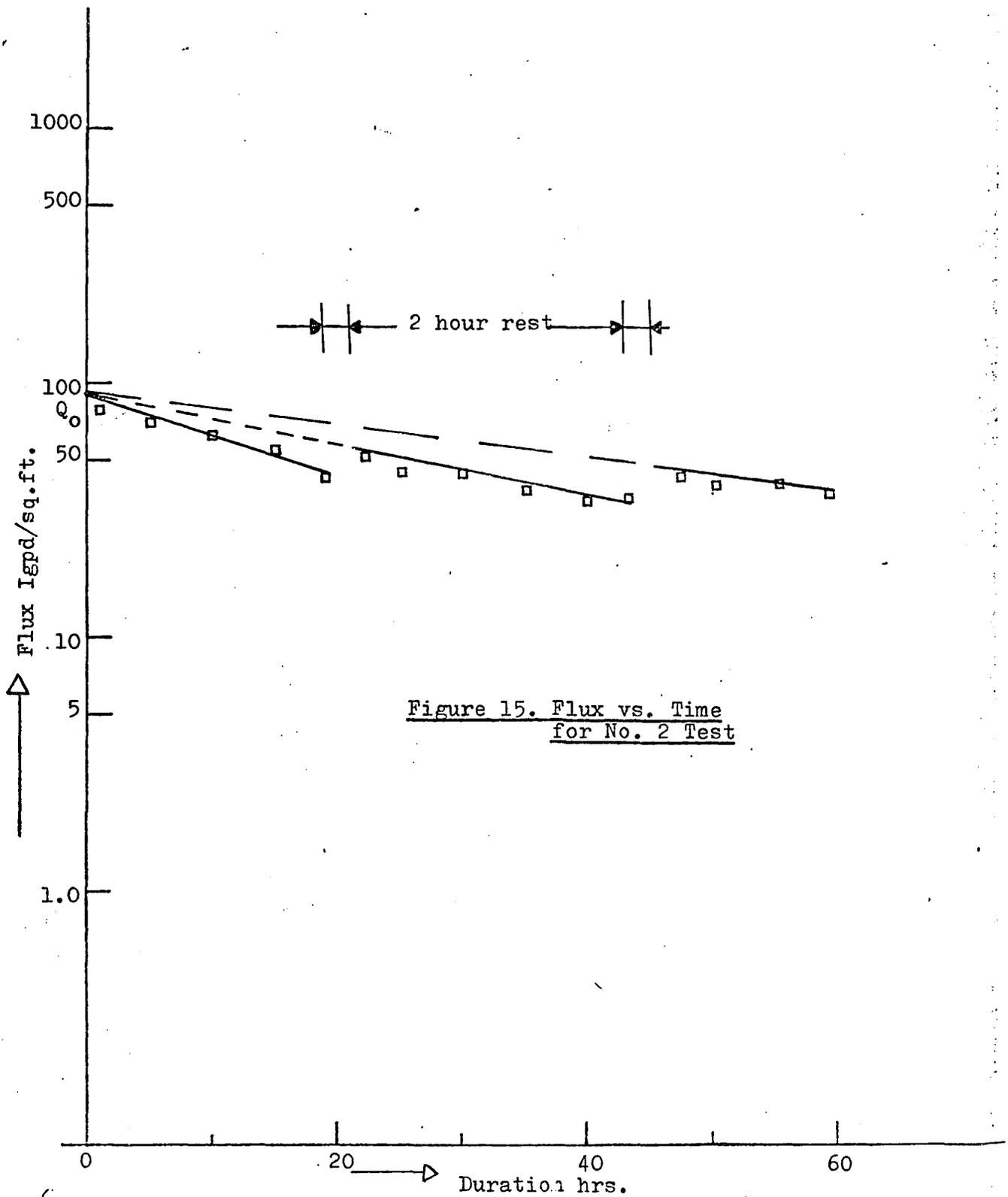
Figure 15. Flux vs. Time
