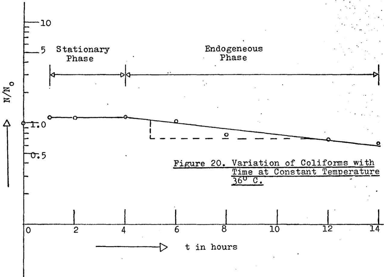
Figure 20. Variation of Coliforms with Time at Constant Temperature 36° C.
