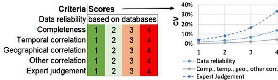
Fig. 2. Uncertainty assessment framework presented in Plank, et al. (2022a) and based on Laner, et al. (2015) where scoring of six criteria is used to assess the reliability of final results and determine a coefficient of variation (CV).
