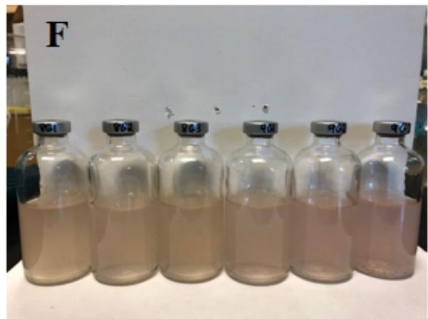
Figure B-3: Images of the reactors after the sequencing batch operation. (A): Controls from left to right, Syntho, Acetate, Starch, Milk and Glycerol. (B): Syntho reactors. (C): Acetate reactors. (D): Starch reactors. (E): Milk reactors. (F): Glycerol reactors.
