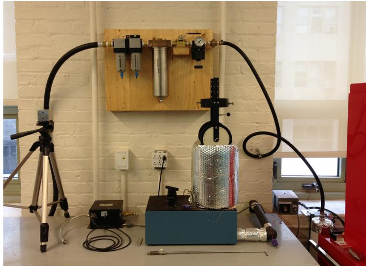
**Figure 2.8:** The laminar calibration jet. Note that the air source and main shutoff valve shown in the schematic below are not seen in the picture.
