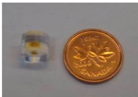
Figure 3–13: The source and scintillator used in the timing probe. The source is in the middle and can be seen as the brown spot.
