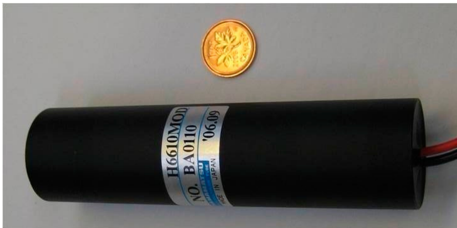
Figure 3–12: The H6610 PMT that is used in the timing probe. Note that the H6610MOD PMT has the same attributes as the H6610 but runs on a positive HV instead of negative HV.
