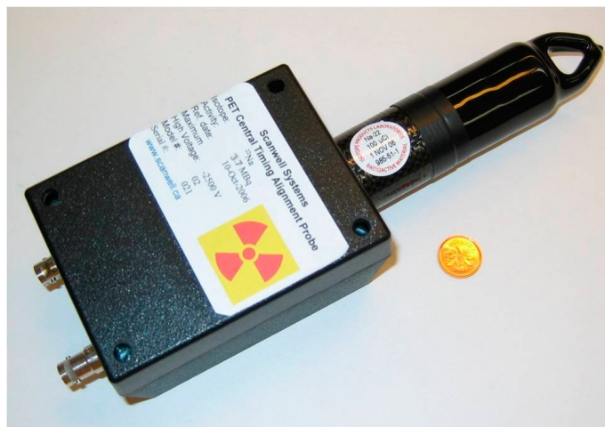
Figure 3-11: New probe with a faster PMT and 10 times the activity of the old probe at manufacturing time (currently the activity is about 20 times higher because of the decay of the sources)
