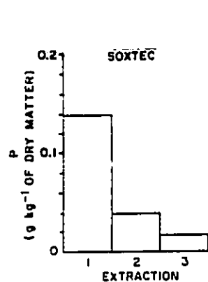
Fig. 5. Phosphorus in each of three sequential 1.5-h ethanol extractions of lyophilized dairy cattle feces by Soxtec. Coefficients of variation (%) were: 1 = 8, 2 = 8, 3 = 4).
