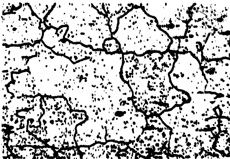
FIGURE 4.31 Pre-strained 12%. Ann. temperature: 715°C. 100 X
