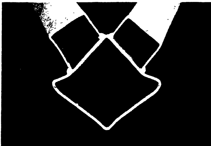
Fig. 2.4 Cross-section distortion. Truss 4.
