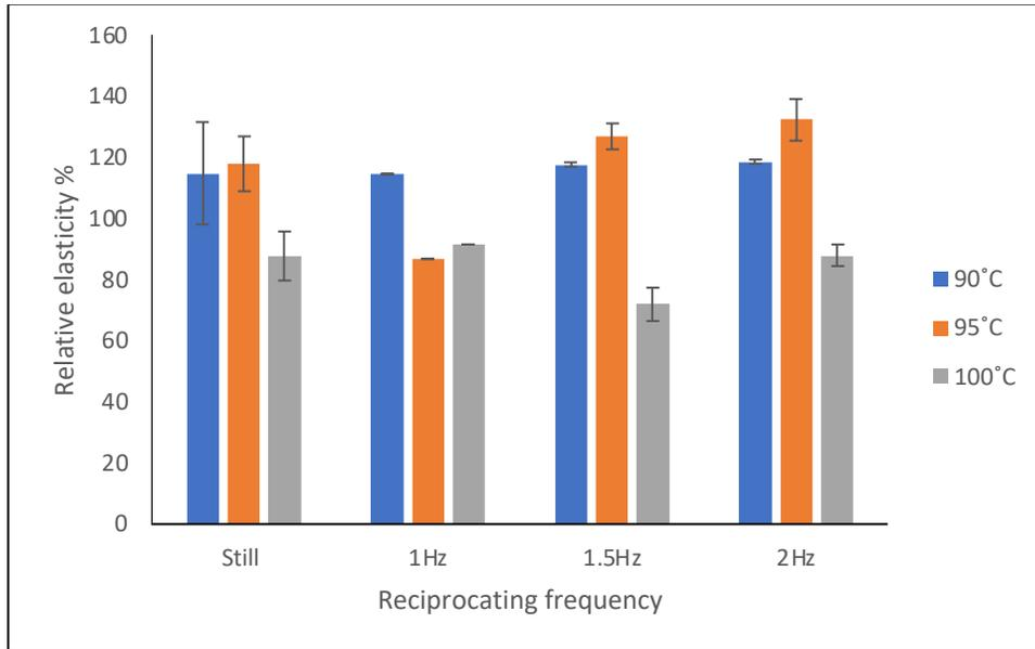
**Figure 4.19. Relative elasticity for peach in RATP**
