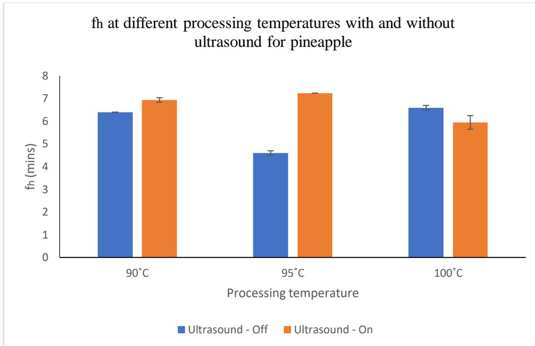
**Figure 3.5.  $f_h$  at different processing parameters for pineapple in USWB**
