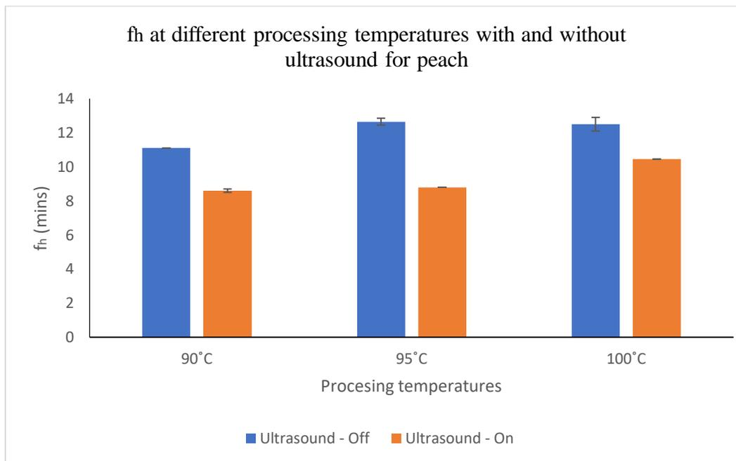
**Figure 3.6.  $f_h$  at different processing parameters for peach in USWB**
