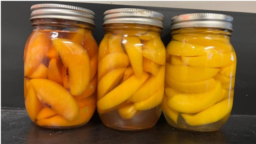
**Figure 4.27. Peach samples processed under still mode at 90°C, 95°C & 100°C.**
