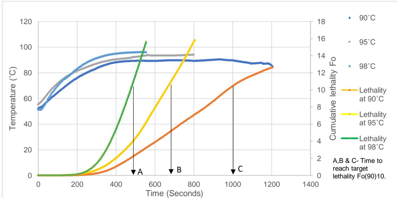
**Figure 3.4. Internal temperature recorded and lethality values obtained for pineapple for USWB**
