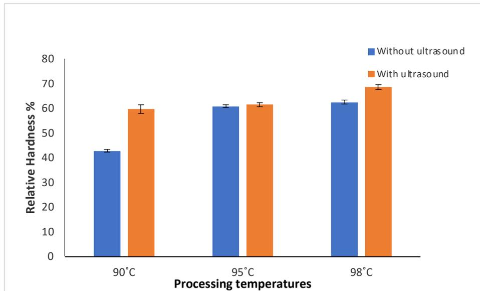
**Figure 4.2. Relative hardness for pineapple in USWB**
