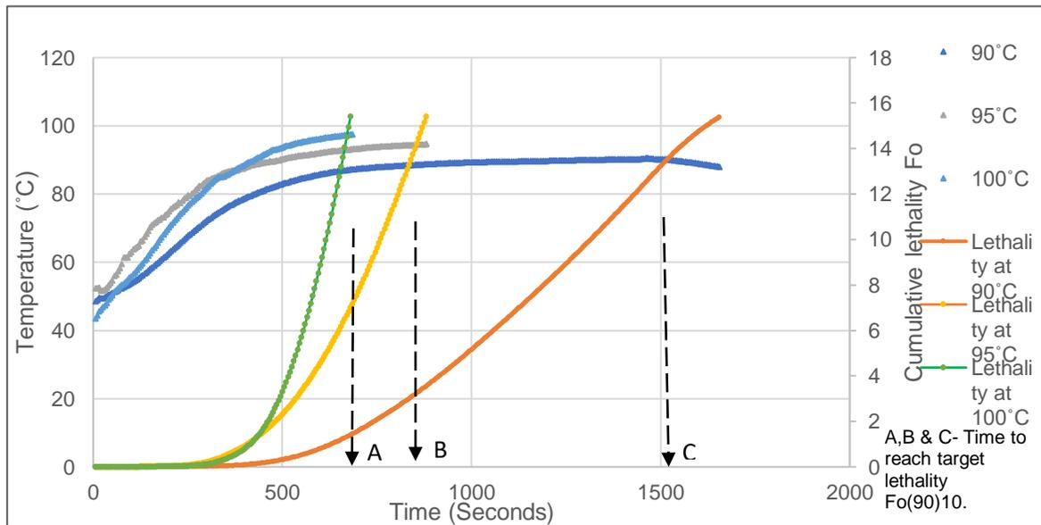
**Figure 3.3. Internal temperature recorded and lethality values obtained for pineapple for RATP**
