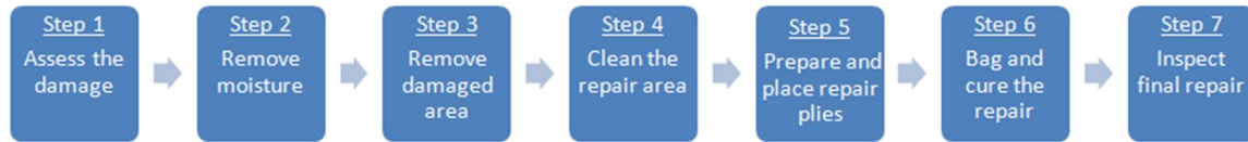
Figure 1-2: Typical in-service repair process flow
