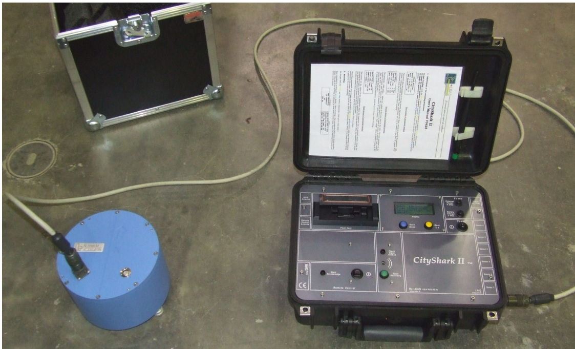
Figure 3.2 CityShark acquisition stations (right) and velocimeter (left)
