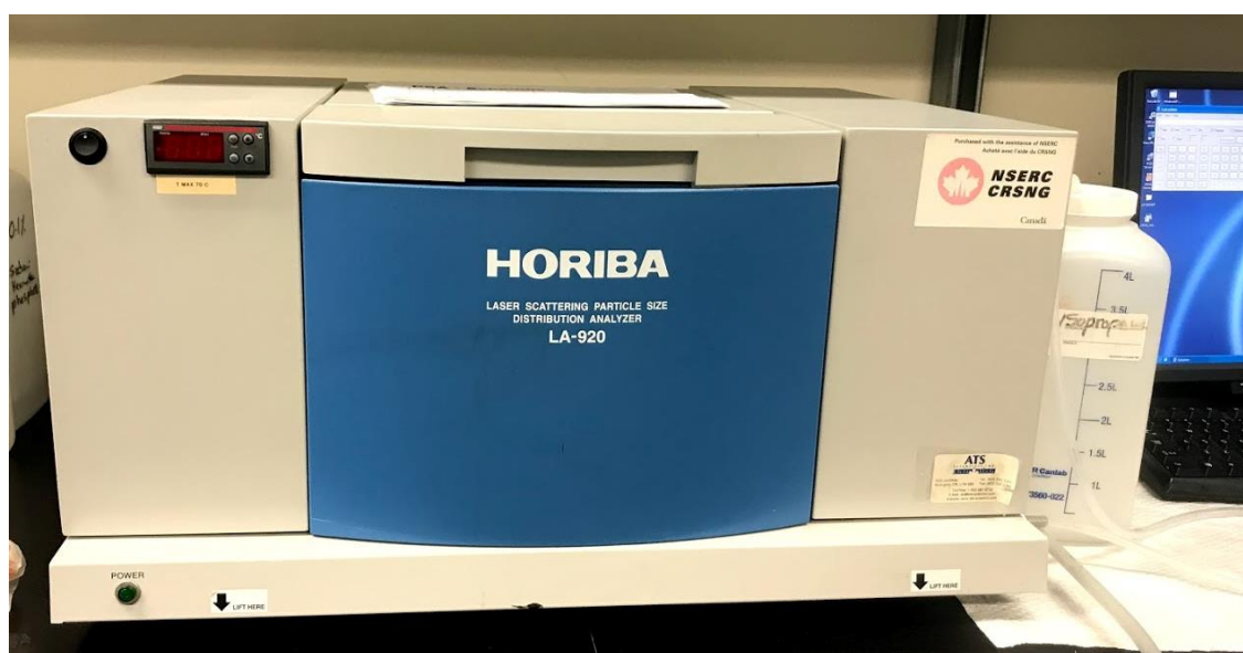
Figure 3.2 HORIBA LA-920 Laser Scattering Particle Size analyzer
