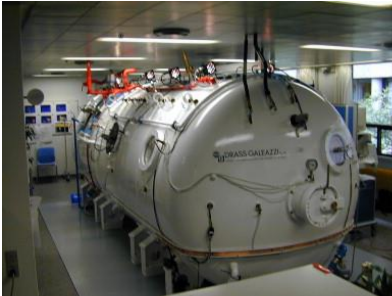
Figure 2-4: Multiplace hyperbaric oxygen treatment chamber. Reproduced with permission from Mortensen. [259]
