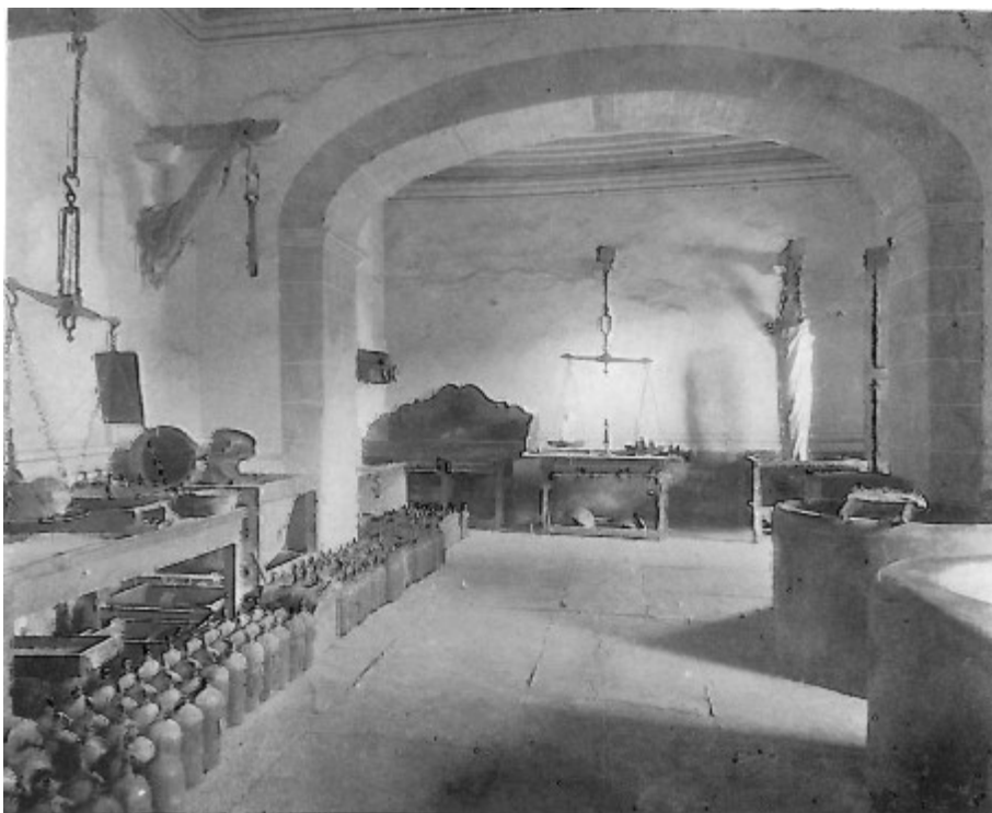
Figure 3-6. Photo of an azoquería (mercury room), showing mercury flasks, scales and vertical white manga held by chains from a beam to the right of the background. Original photo from footnote 435.
