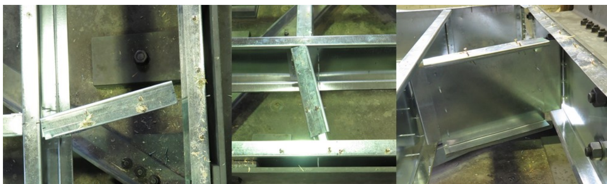
Figure 3.11: Post-Test Blocking Connections along Fixed End (Damage)
