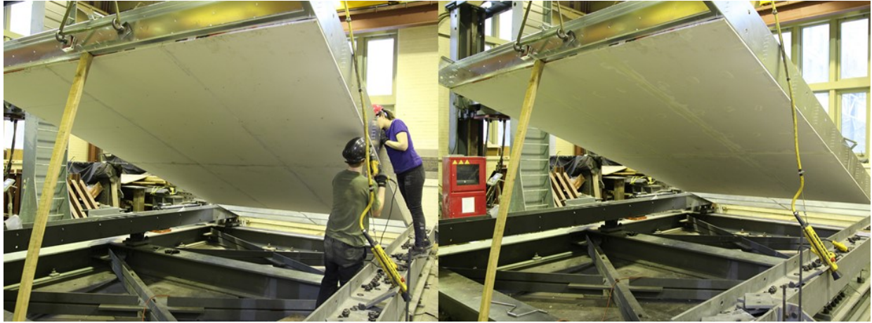
Figure 2.9: Specimen 14-RGY-P-M Before and After Joint Tape and Compound was Placed Between Panels and at Screw Locations
