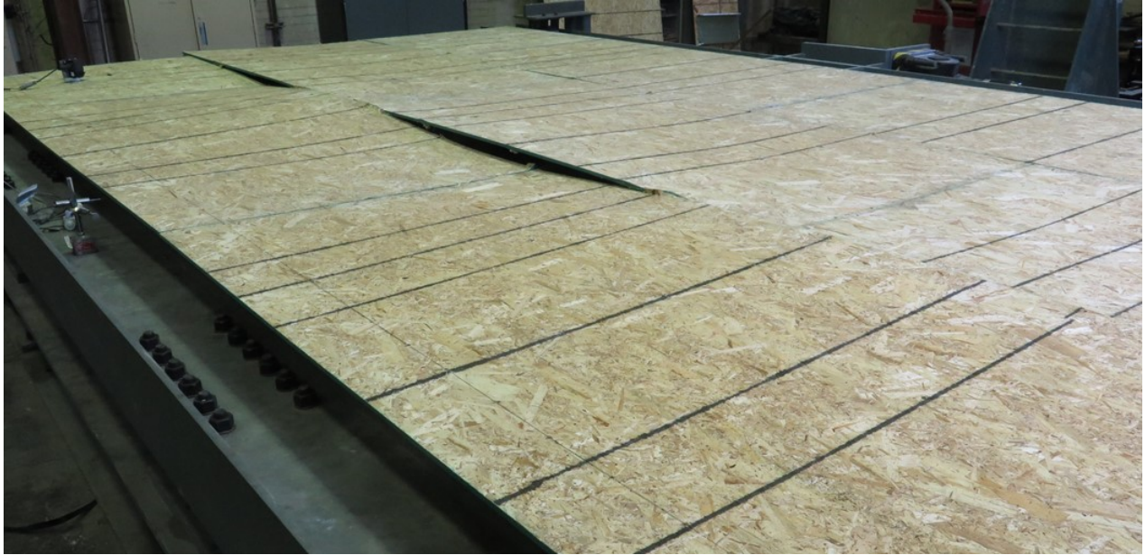
Figure 3.24: Lift Off of OSB Panels After Failure of Sheathing Fasteners
