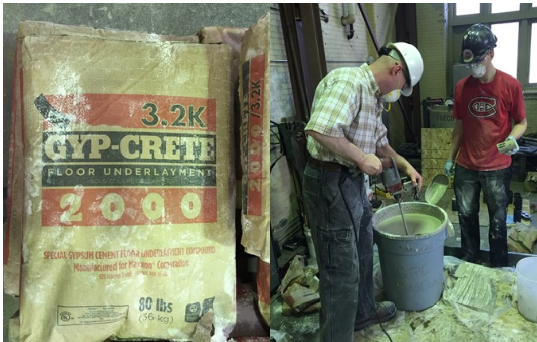
Figure 2.23: (Left) Photo of GYP-CRETE2000®/3.2K (Right) Photo of Barrel Batch Mixing Process
