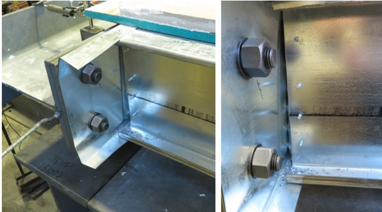
Figure 3.33: Extensive Deformation at North-East Joist – Rim Joist Connection
