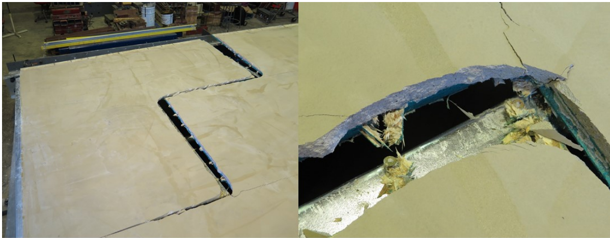
Figure 3.35: Tension Fracture of Gypcrete Topping with Tear out Failure of Sheathing Fasteners
