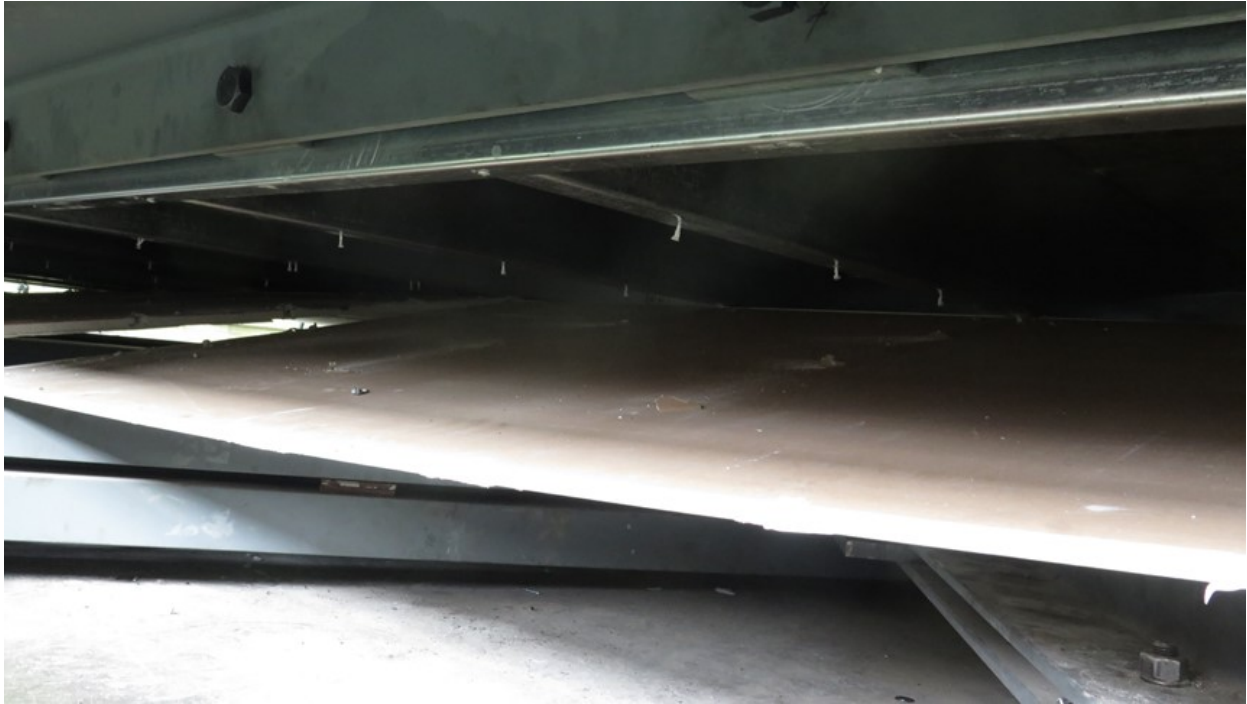
Figure 3.30: Connection Failures of Gypsum Panels for Specimen 15-RGYP-C
