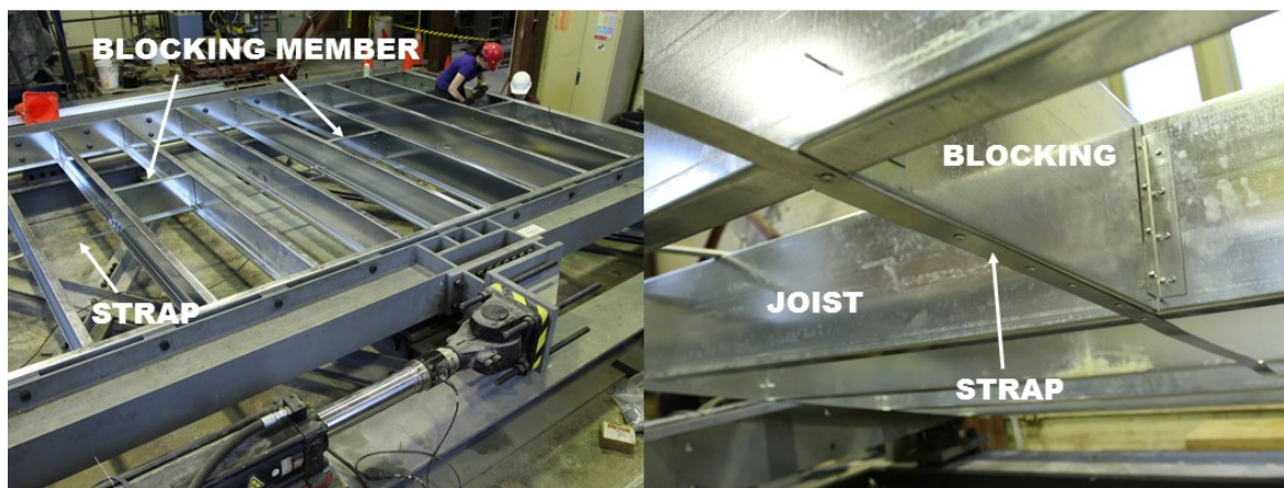
Figure 2.15: (Left) Unblocked Specimen (14-RGYP-M) (Right) Web-Stiffener to Joist Connection (Closed Face)
