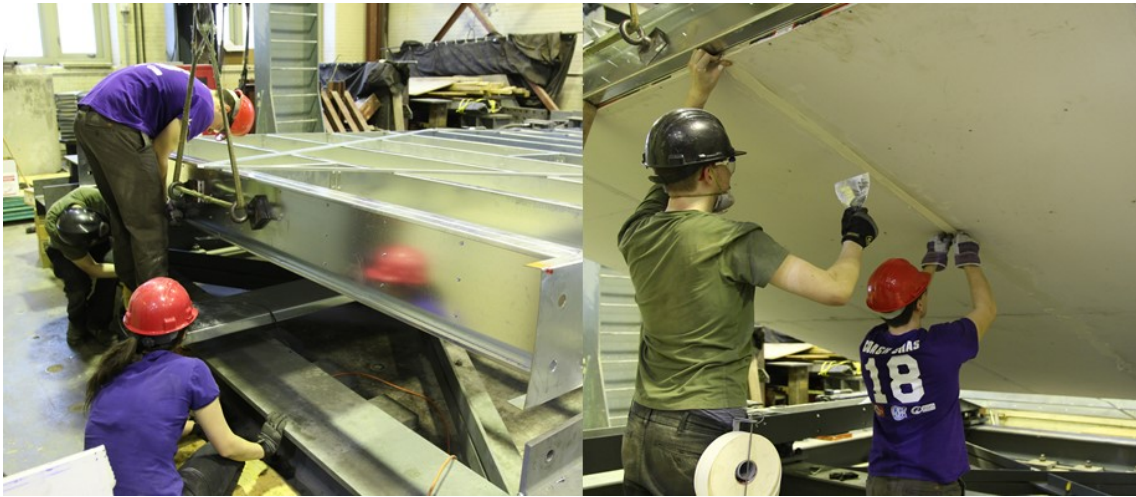
Figure 2.21: (Left) Initial Lift of Specimen 14-RGYP-M Using I-Hooks (Right) Applying Joint Tape and Compound to Panel Interface
