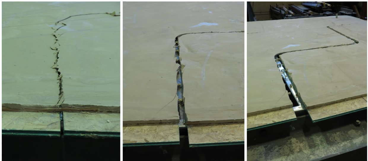
Figure 3.34: Separation of Panels with Increased In-plane Displacement (Post-Peak Loading)
