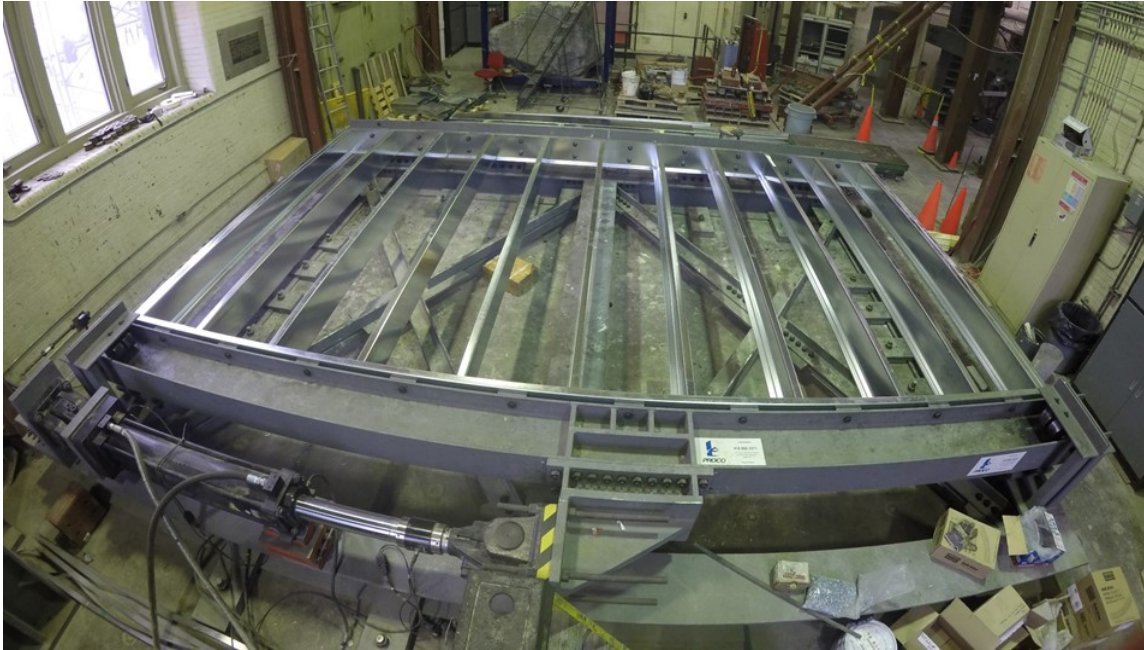
Figure 2.14: Diaphragm Specimen After Installation of Rim Joists and Joists
