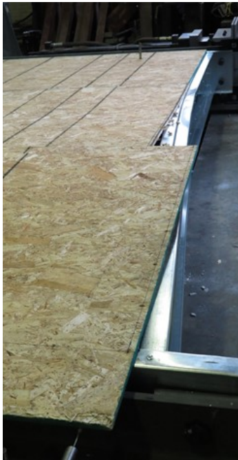
Figure 3.25: (Left) Displacement of Sheathing and Bending of Double Joist (Right) Tear-out of Sheathing Fasteners and Gypsum Failure
