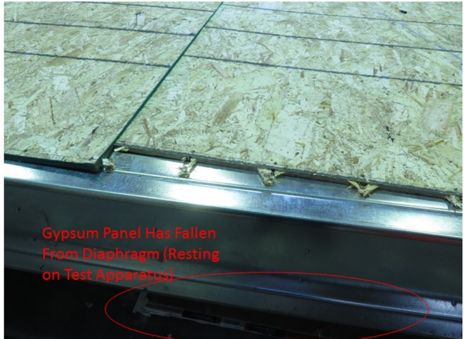
Figure 3.25: (Left) Displacement of Sheathing and Bending of Double Joist (Right) Tear-out of Sheathing Fasteners and Gypsum Failure
