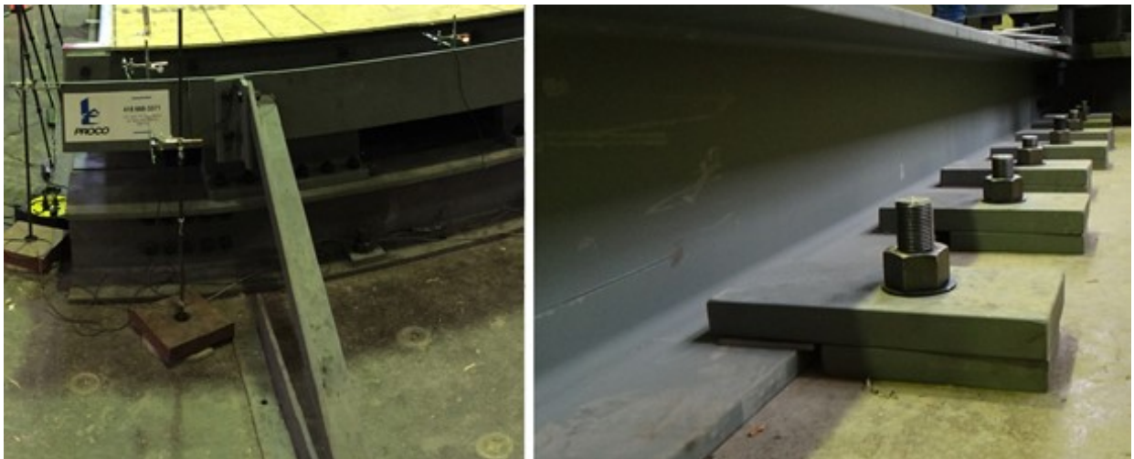
Figure 2.4: (Left) Fixed End Connection (Right) Pre-Tensioned 38mm Threaded Rods
