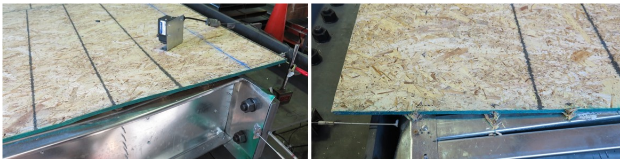
Figure 3.9: Sheathing Failure along Fixed End of 11-RALT-M
