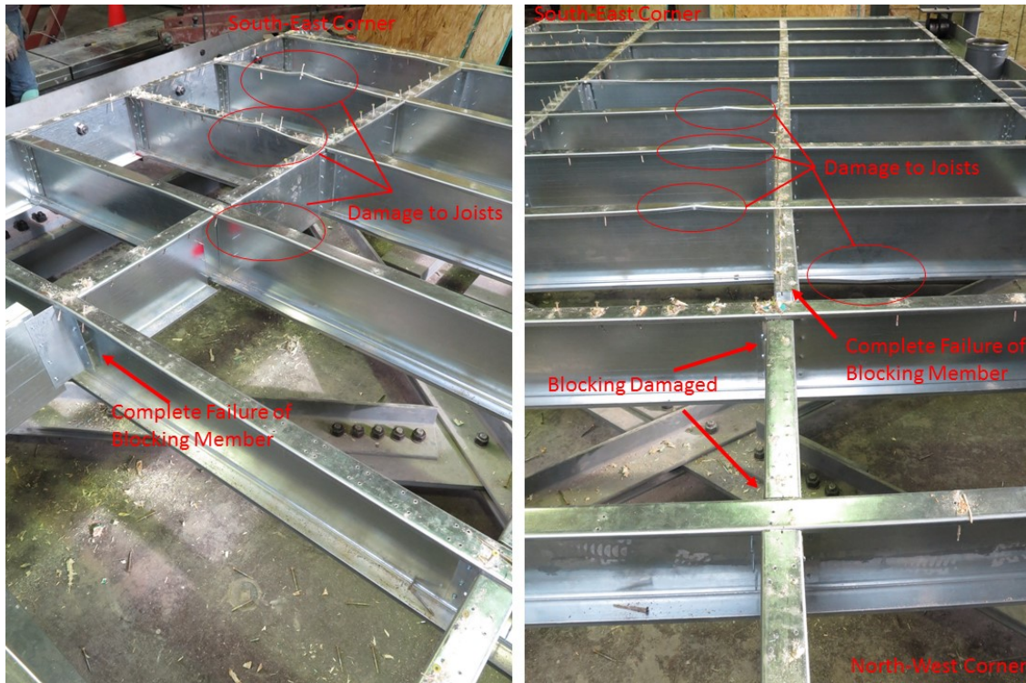
Figure 3.22: Damage to Frame Members of Specimen 13-FB4-M Caused by Compression Field in CFS Structure
