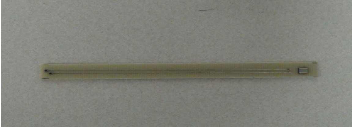
Figure 15: Wired bonded inter-digitized electrode
