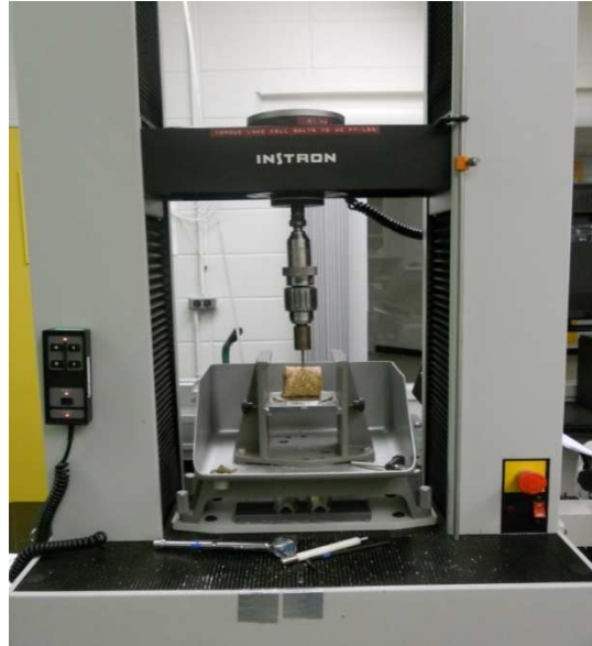
Figure 5.3 Instron setup for puncture test of firelogs
