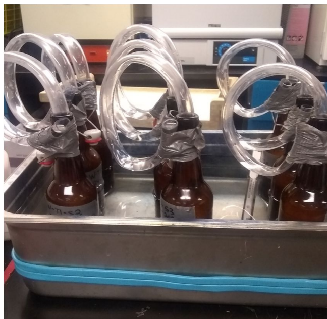
Figure 1. Experimental set-up for SSF: individual sample bottles fitted with plastic tubing airlocks, sitting in heated water bath
