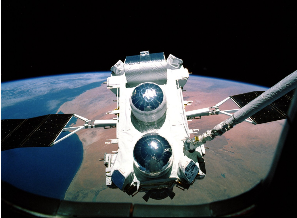
Figure 1.4: The Compton Gamma-Ray Observatory being deployed from the Space Shuttle Atlantis with the aid of the Canadarm (April 1991). The reflective outer surfaces of the detectors helped to maintain thermal equilibrium. In addition to the pair-production telescope EGRET (situated in the lower dome in this view), there were three other instruments which were sensitive only at energies \lesssim 0.1 GeV: the Burst And Transient Source Experiment (BATSE); the Oriented Scintillation Spectrometer Experiment (OSSE); and the Imaging Compton Telescope (COMPTEL). The BATSE array was distributed across the eight corners of the satellite platform; OSSE had four independent detectors housed in the box at the top; and COMPTEL resided in the central dome. Image credit — crew of STS-37, Compton Science Support Center, NASA.
