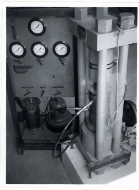
Figure 4-8 (b): Triaxial testing apparatus.
