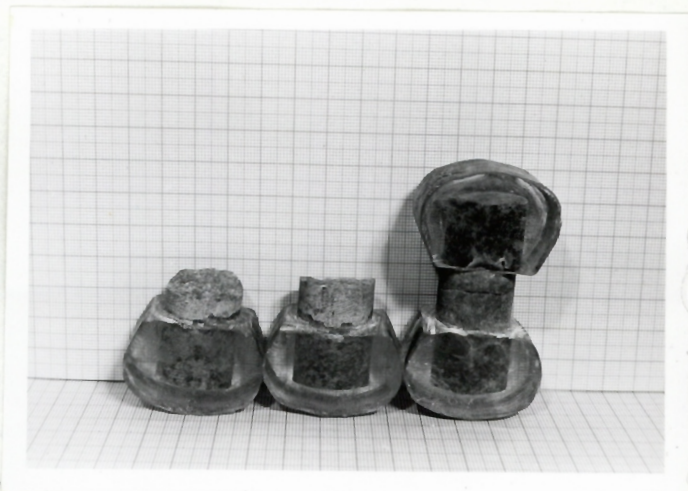
Figure 5-7: Clean breaks by pull test. Specimen PA-15 and PA-33.
