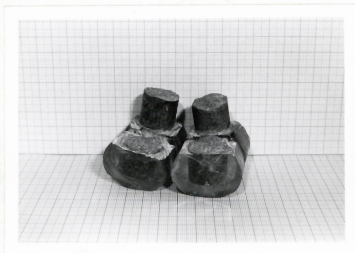
Figure 5-8: Doubtful breaks by pull test. Specimen PB-8 and PB-22.
