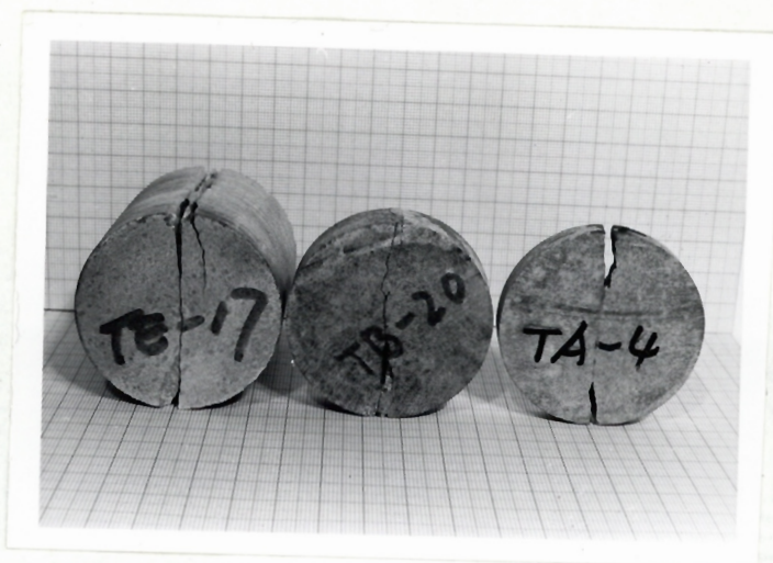
Figure 5-13 : Tensile failure, Brazilian test. Specimens TA-4, TB-20, TE-17.
