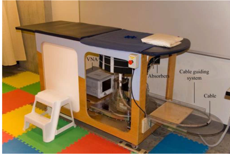
Figure 2.9. A photograph of the TSAR system from [40]. Certain components, VNA, EM absorbers, the cable guiding system for the moving antenna, are labelled in the photograph.
