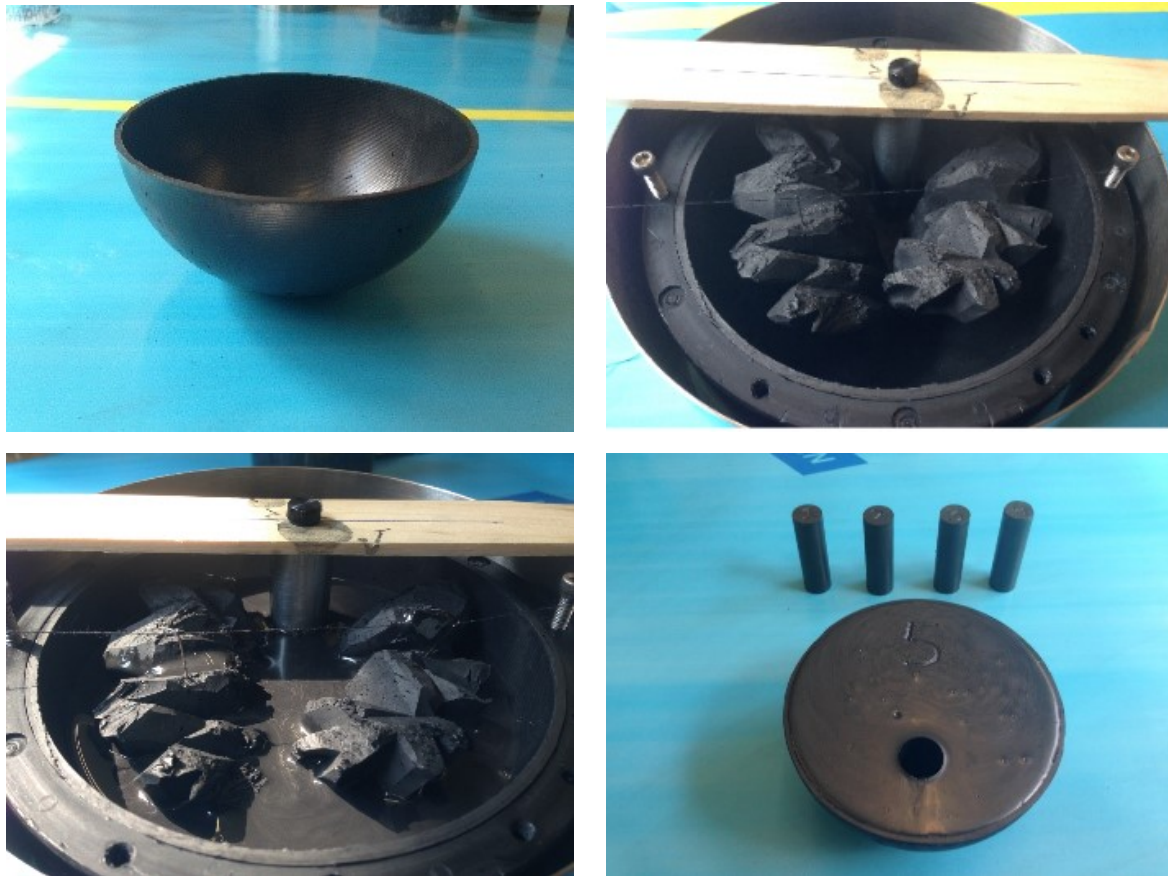
Figure 4.5. A set of four images depicting the phantom fabrication process (clockwise from top left): empty skin, placement of glandular structures, filling the breast with adipose tissue while maintaining a spot for the plug, and a complete phantom with several plugs, [104].
