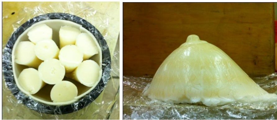
Figure 3.5. An example of the heterogeneous breast phantoms. (Left) A photograph of the 2-mm skin layer and the conical gland structures embedded inside the phantom. (Right) An example of the realistically shaped breast phantom, exterior only [64].
