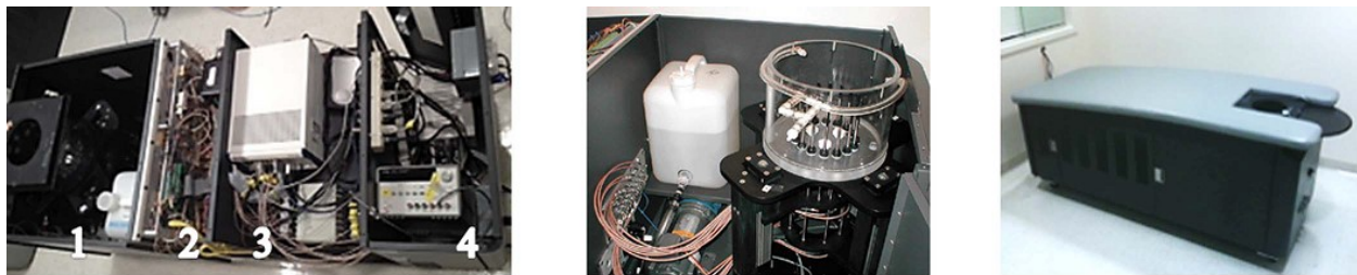
Figure 2.8. Photographs of the system components from [38]. (Left) The system’s main compartmentalized components: 1 – Interface between the immersion tank and liquid, 2 – the microwave electronic networks, 3 – the data acquisition components, 4 – the power supplies. (Middle) The immersion tank and antenna array, attached to the liquid reservoir and the microwave electronic network. (Right) The complete system as it appears in the clinic.
