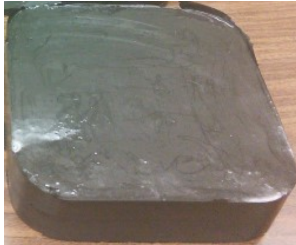
Figure 4.10. A photograph of the finalized large scale rubber phantom. There are four inclusion embedded within the phantom.
