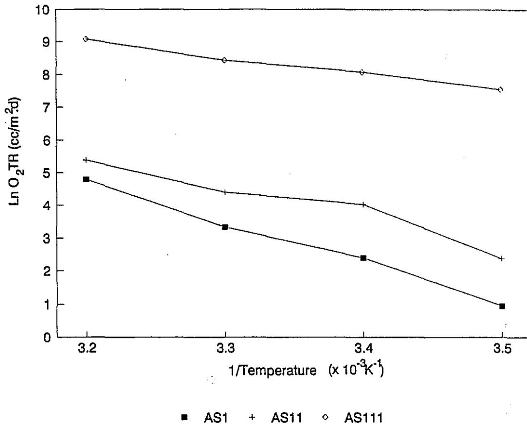
Figure 30 Arrhenius plot of oxygen transmission rate versus temperature change
