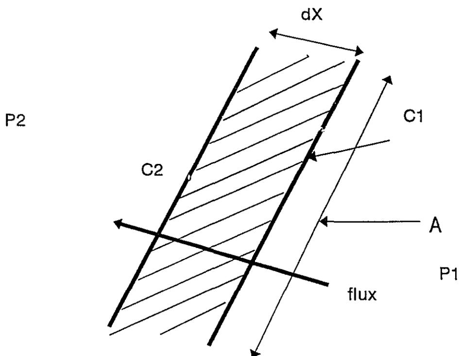
Figure 29. Schematic representation of "activated diffusion" across a packaging film.
