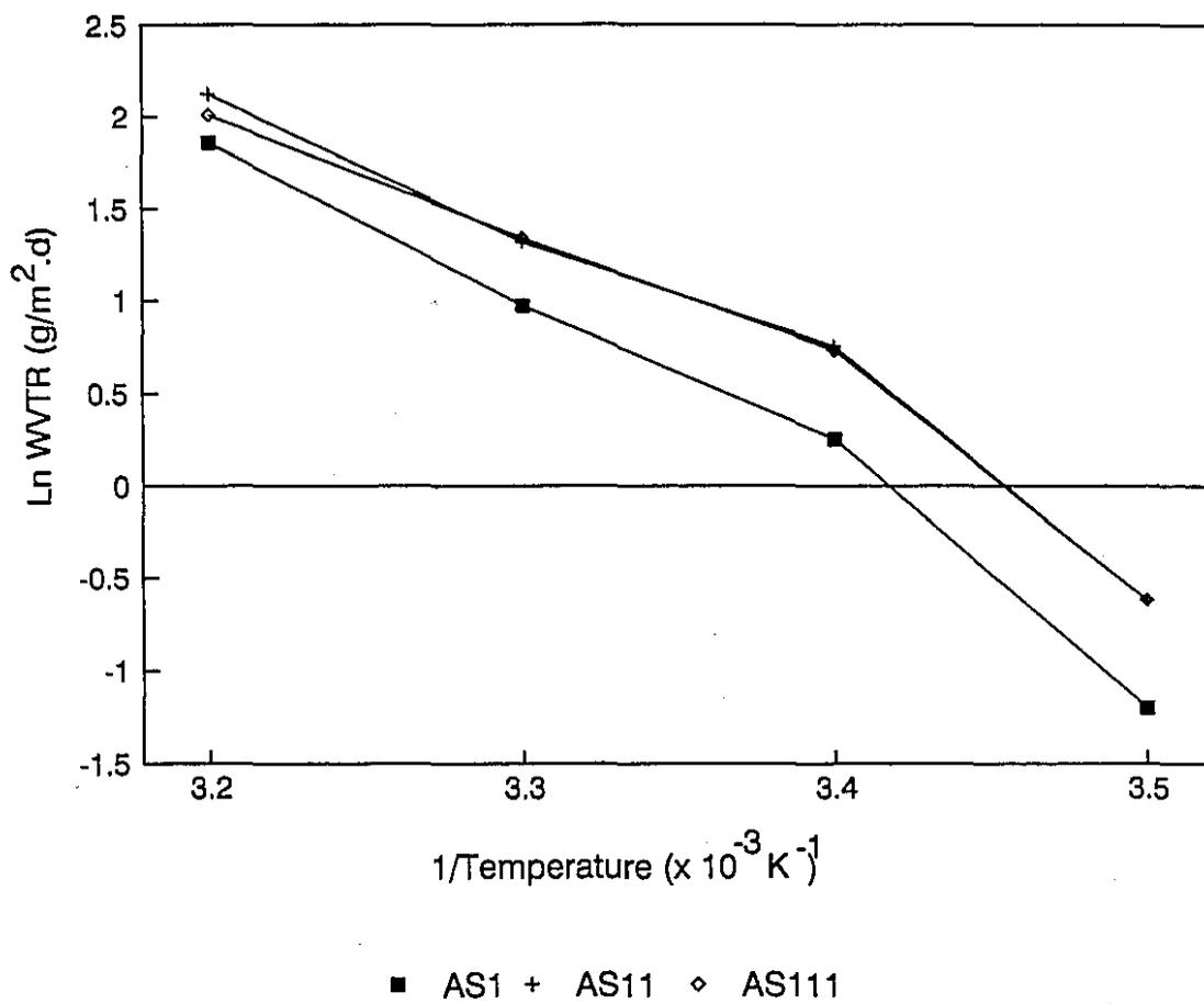
Figure 32 Arrhenius plot of water vapour transmission rate versus temperature changes
