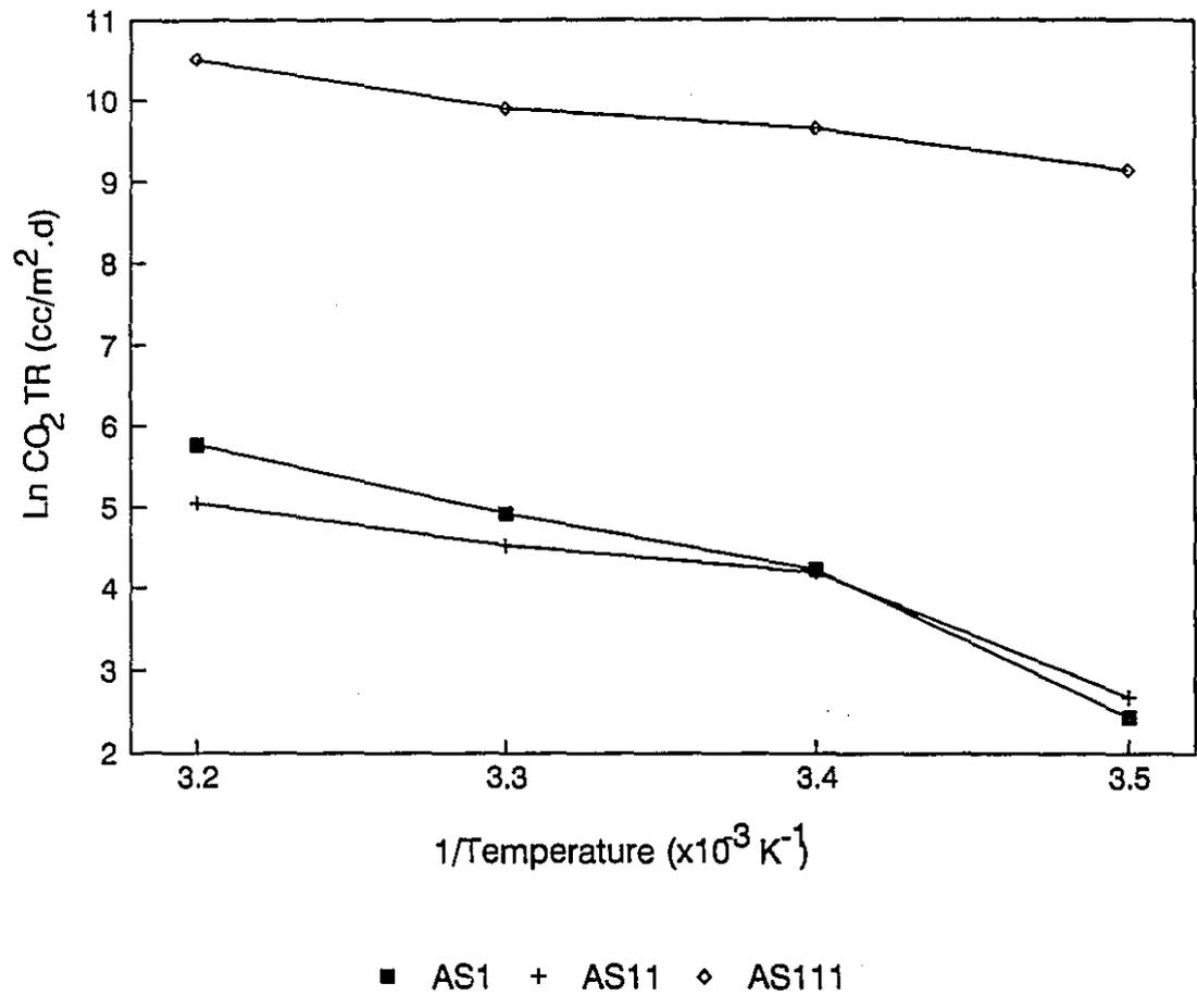
Figure 31 Arrhenius plot of carbon dioxide transmission rate versus temperature change
