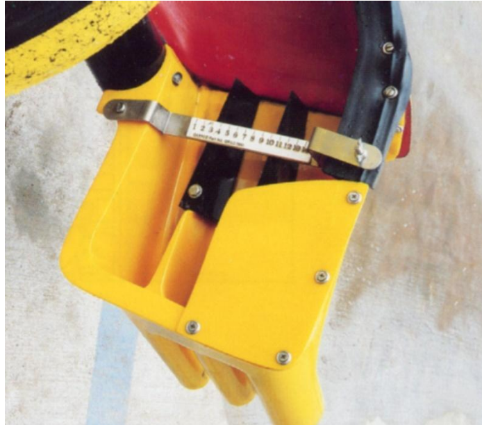
Figure 3 - The splitters of a spiral concentrator (Mine-Engineer.Com, 1994-2012)
