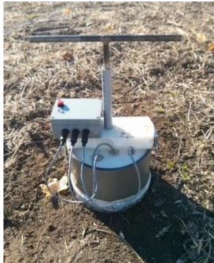
Figure 3.2: Picture of the first RSCA prototype using a built-in piston system
