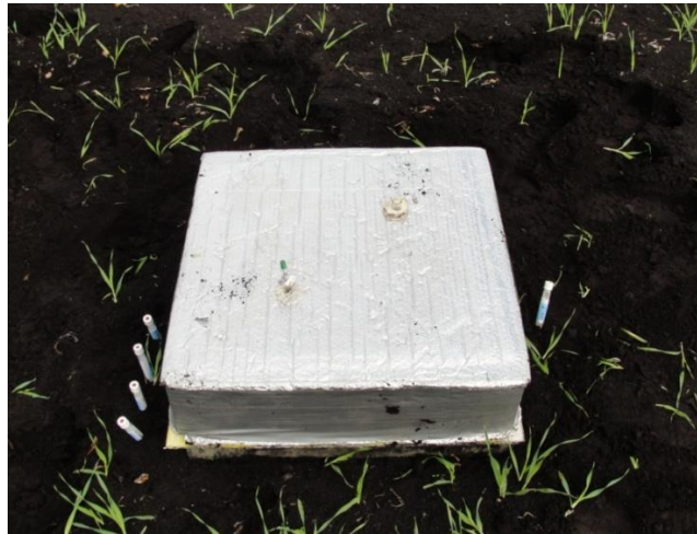
Figure 3.13: Picture of non-steady state chamber and exetainers used for gas sampling, by Mat-Su (2016)
