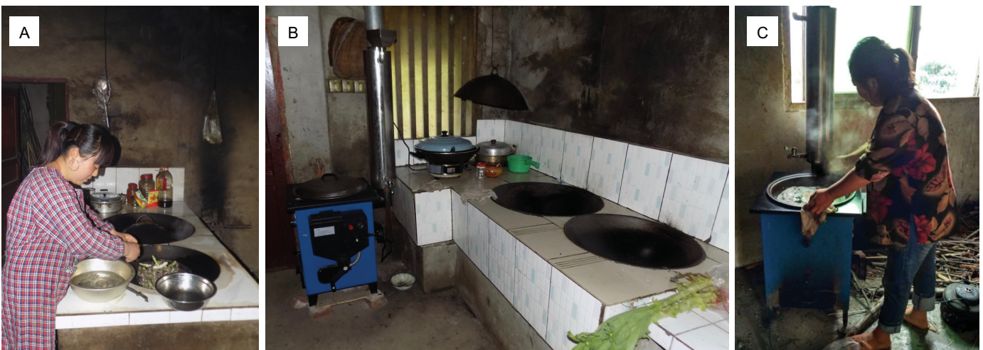
Figure 1. Traditional biomass chimney stove and semi-gasifier cooking and water heating stove in study kitchens. In Plot A, a woman is frying vegetables on a traditional chimney stove;
