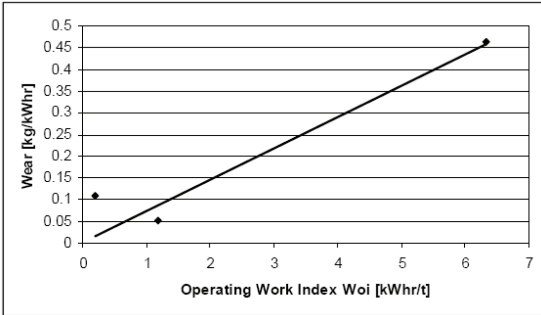
Figure 3.2: Wear vs. operating work index (Radziszewski, Hewitt et al. 2008).
