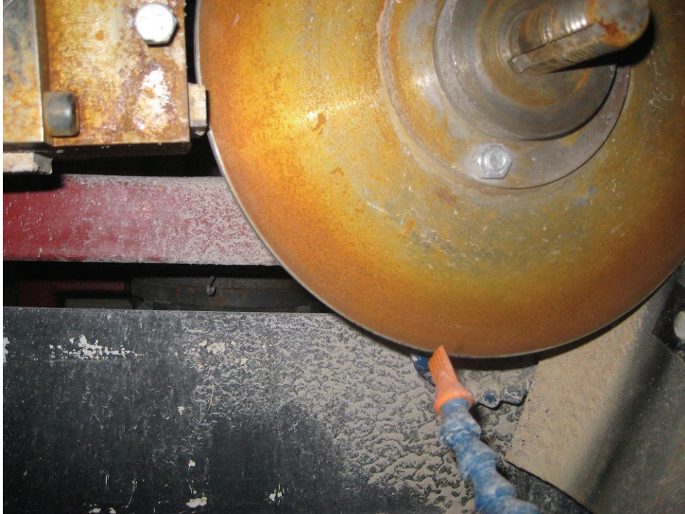
Figure 7.2: New water flushing system used for wet tests.
